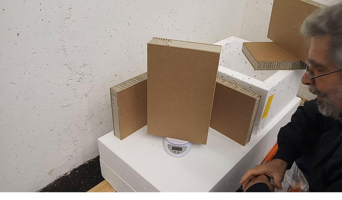
400 mm x 240 mm x 50 mm = 406 g = 84 kg / m<sup>3</sup> 400 mm x 240 mm x 70 mm = 567 g = 84 kg / m<sup>3</sup>
